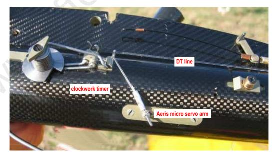
Example of a simple DT release mechanism in a F1C model The DT line is released either by the timer or by the *Aeris* SA micro servo
